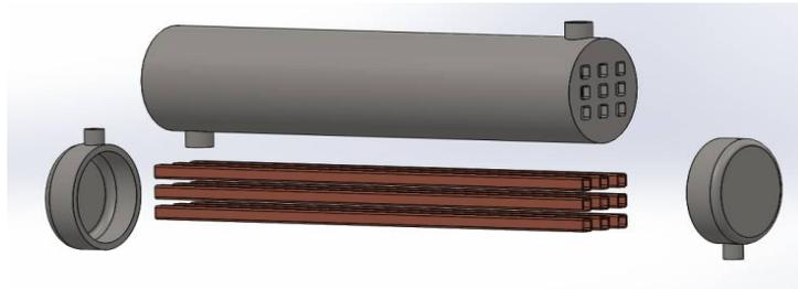
Fig 4: Square with fillet c/s tube Heat Exchanger model
